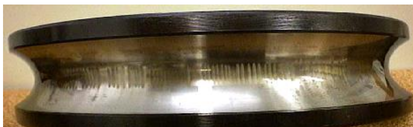
Figure 18 – ‘Characteristic ‘fluting’ wear of inner race
