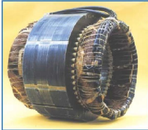
**Figure 18 Completed random winding**
