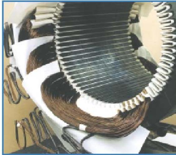
**Figure 16 Partially wound stator core with random winding**
